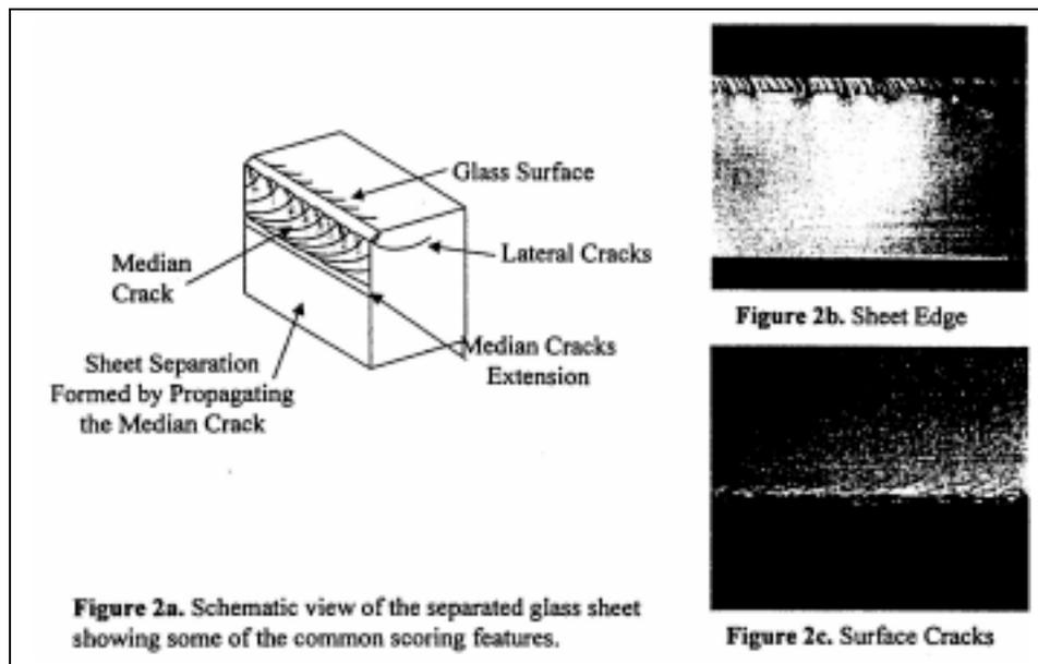
The contoured surface on the median crack surface is created as score wheel wedges the crack open. The wheel tip surface finish and tool wobble account for most of the markings. The wheel tip's non-uniform ground surface, the primary contributor, turns the crack by pushing on alternate sides of the crack face. In Figure 2, the score wheel has run from left to right.
