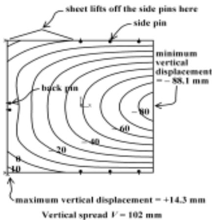
when the back edge is supported, the downward vertical displacement reduces in magnitude, but the two back corners of the sheet lift upward, so the vertical spread remains roughly the same. The two pins supporting the back edge in Figure 2 are spaced 50 mm apart. Increasing the spacing, or using more pins, does not help either; the vertical spread remains about the same.
