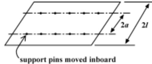
For **two rows** of support points, the optimal separation between the rows that gives the least vertical spread has<sup>2</sup>
