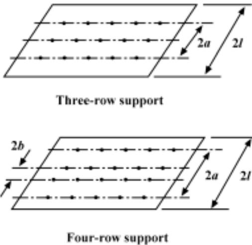
From the preceding formulas, for a 2000 mm x 2000 mm x 0.5 mm sheet of Corning 1737 glass, the vertical spread is about 12 mm under optimal three-row support, and about 3.5 mm under optimal four-row support. Both those values of vertical spread are within acceptable limits.
