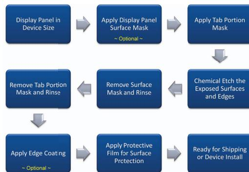
Figure 7. General process flow for strengthening a device level display panel.
