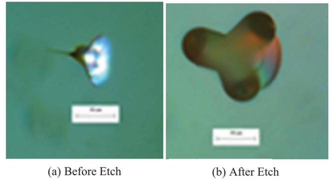
Figure 2. Three gram indents before (a) and after (b) etching.
