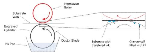
Fig. 3 Basic principle and arrangement of the components for gravure printing.
