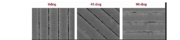
Fig. 6 Comparison of gap quality of 50  $\mu\text{m}$  nominal gap for nanosilver ink printed at three different angles to print direction.
