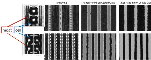
Fig. 7 Comparison of printability of 200  $\mu\text{m}$  nominal line by using two different engraving approaches.
