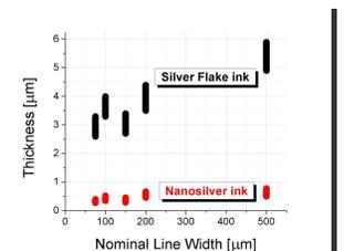
Fig. 11 Comparison of line thickness range for different nominal line widths for the two conductive inks.
