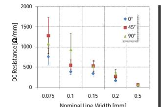
Fig. 9 DC resistance values for resistors with different nominal line widths for nanosilver ink printed at three different angles to print direction.
