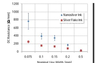
Fig. 8 DC resistance values for resistors with different nominal line widths for two conductive inks printed (lines printed in parallel to print direction, 0°).
