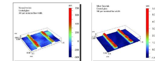
Fig. 10 The 3D images of 100  $\mu\text{m}$  nominal line printed with nanosilver ink (left) and silver flake ink (right) on glass substrate (measured by a vertical scanning interferometry (VSI) using a WYKO RST-Plus microscope).
