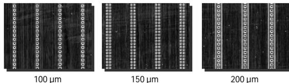
Fig. 2 Engraving for traces with different nominal width. (Images taken with ImageXpert Image Analysis System at 40x magnification)
