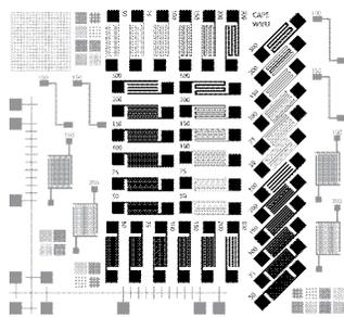
Fig. 1 Section of printing design (meander lines and lines with different spacing (gaps) at 0, 45, 90° to print).
