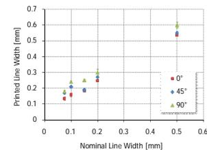
Fig. 4 Comparison of printed vs. nominal line width in print direction for two conductive inks printed on glass substrate.
