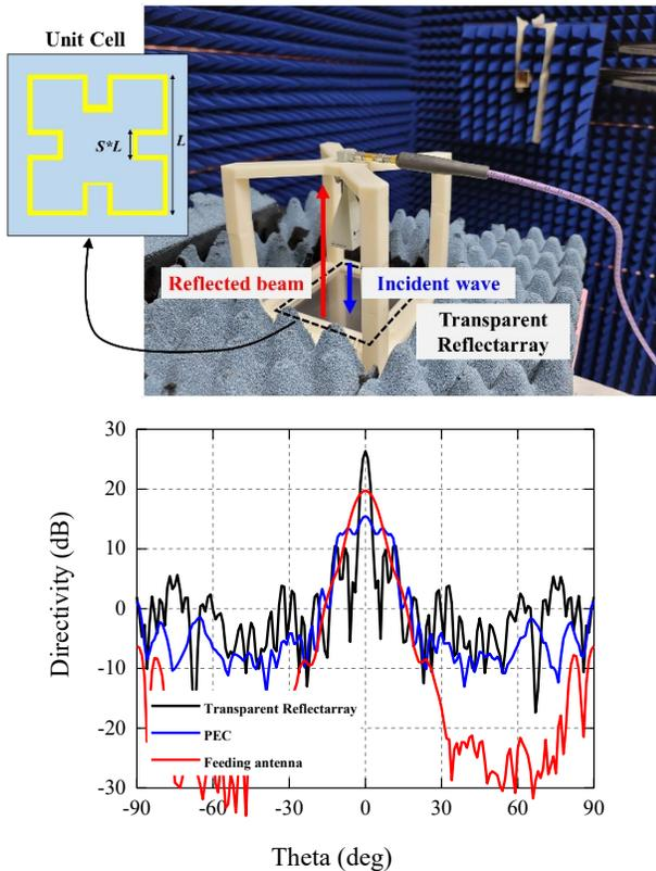
**Figure 4. Display-integrated reflectarray configuration and directivity enhancement of reflected beam.**
