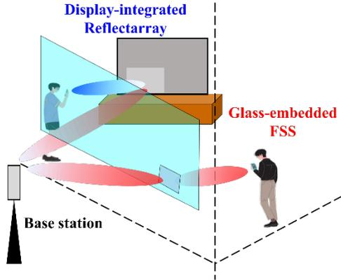
Figure 1. Application scenario of the glass-embedded electromagnetic surface.
