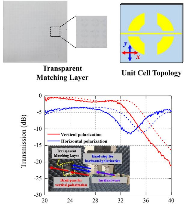
Figure 3. Transparent impedance matching FSS featuring frequency- and polarization-selective responses. (solid: measurement), dotted (simulation).
