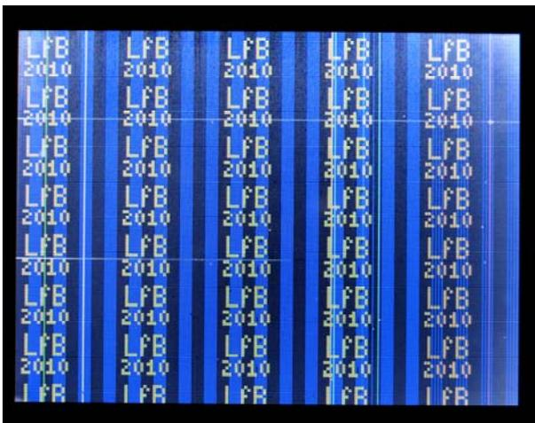
**Fig. 8. Working AM-LCD prototype on ultra-thin glass**
