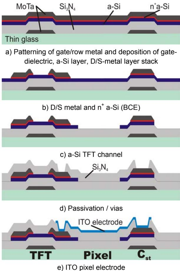
Fig. 1. Five mask a-Si backplane process
