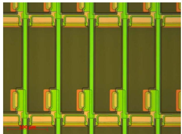
Fig. 3. Completely fabricated ultra-thin glass backplane
