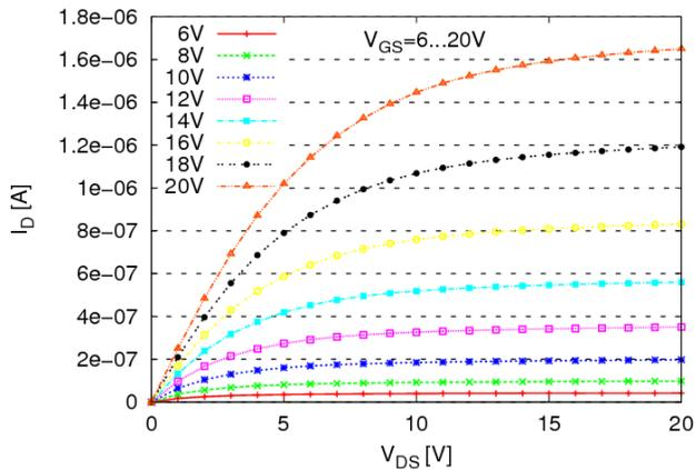
**Fig. 7. Output characteristics of test-TFTs**
