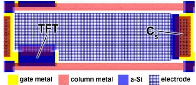
Fig. 2. Lateral design of a single pixel
