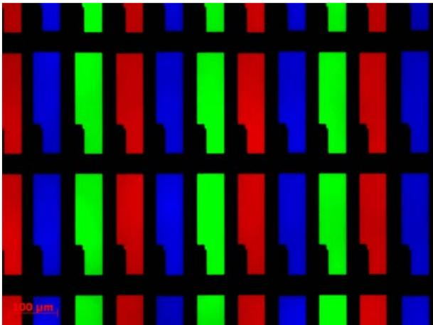
**Fig. 4. Color filter with black matrix on ultra-thin glass**
