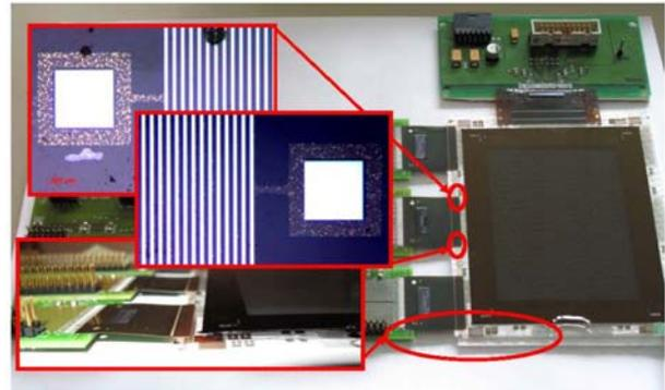
**Fig. 5. Display with precise bond connection / MoTa (white) on Au contacts of TAB**
