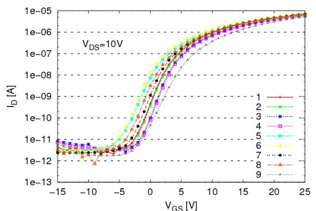
**Fig. 6. Transfer characteristics of test-TFTs**
