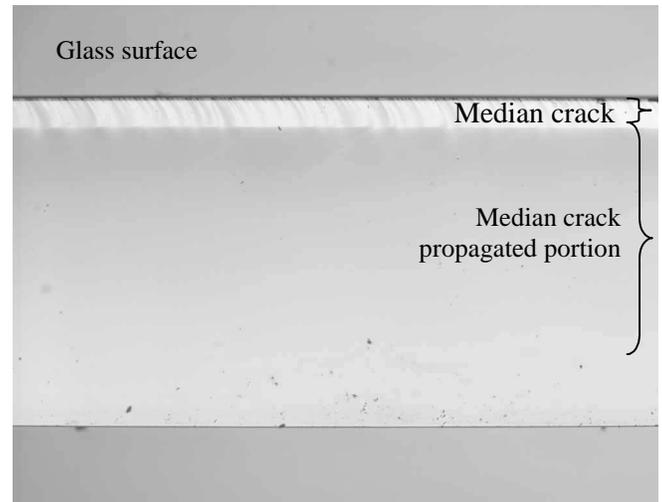
Fig. 14 Typical fracture surface by good cutting. Median crack depth is stable, and the median crack propagated portion is smooth.
