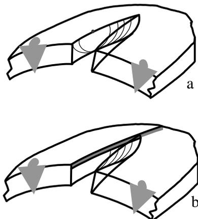
Fig. 13 Schematic illustration of (a) breakage and (b) cutting. The only difference between (a) and (b) is the origin of crack propagation. Irregularly created damage as origin for breakage (a) and median cracks created with scribing as controlled origin for the cutting (b).
