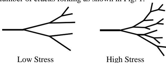
Fig. 1 Forking with high and low stresses
