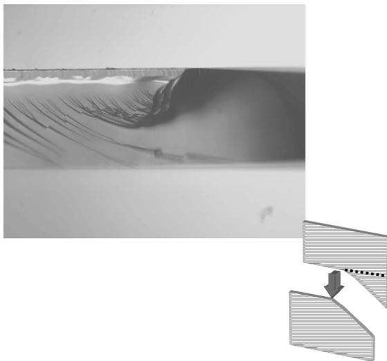
Fig. 15 Fracture surface of miss-breaking sheet by inappropriate separation [13].
