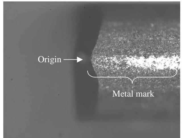
Fig. 11 Around the origin. This picture was taken from apex of the ground edge. Vertical axis in this picture is thickness direction.
