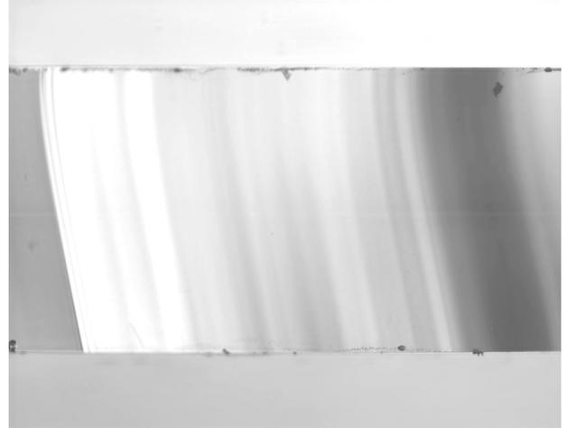
Fig. 9 Wallner lines on fracture surface Thermal stress is one stress that can generate this shape of Wallner lines. The crack runs right to left.
