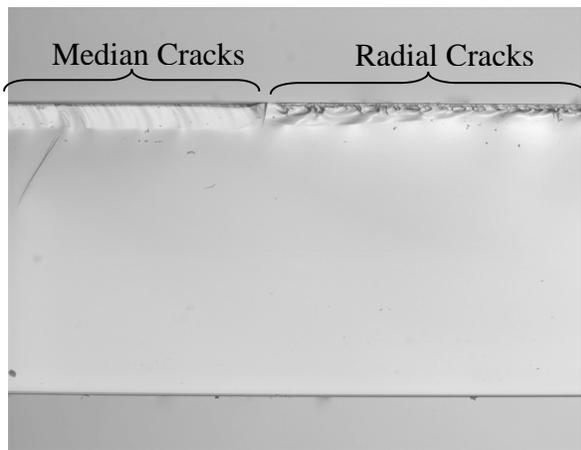
Fig. 16 Cut surface where the median crack stopped. Scribe wheel runs left to right.
