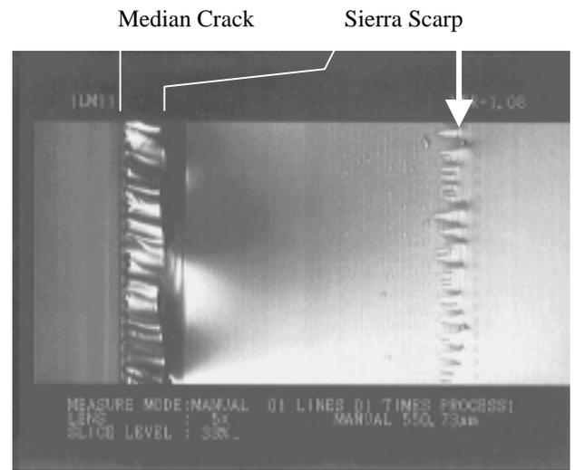
Fig. 7 Sierra Scarp appears on a fracture surface created by scribe/break process. Water was present during median crack propagation.
