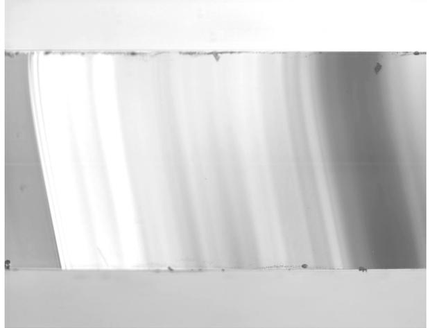
**Fig. 9. Wallner lines on fracture surface
