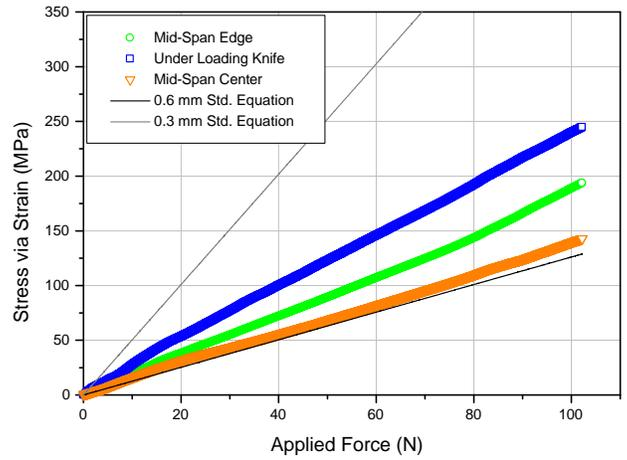
Figure 3. Strain Gage Results with Standard Equation.
