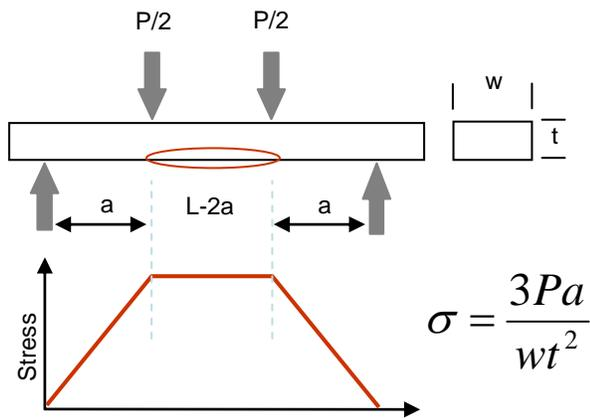
Figure 1. Four-point Bend Schematic with Equation.
