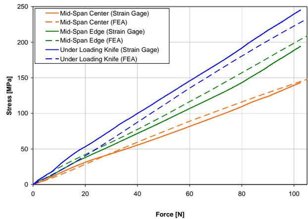
Figure 4. Force to Stress Comparison of FEA Model and Strain Gage Results.
