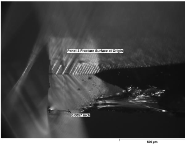
**Figure 5. Break Origin with Mirror Measurement.**
