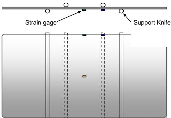
Figure 2. Four-point bend schematic of panel with strain gage locations.
