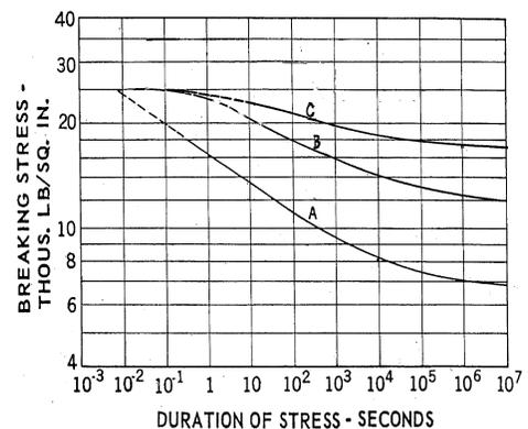
Figure 2. Strength loss due to fatigue [5] (A) soda-lime glass; (B) borosilicate glass; (C) fused silica glass.
