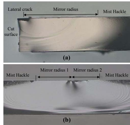
**Figure 7. Typical fracture pattern when surface-4 is seen under a microscope (fracture was initiated from surface-4) (a) Failure origin on the edge; (b) Failure origin on the surface.**
