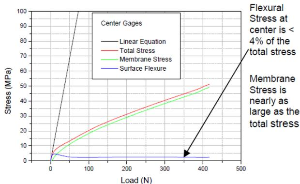
**Figure 3. Not accounting for large deflections can result in estimated stress to be off by a significant amount [6] .**
