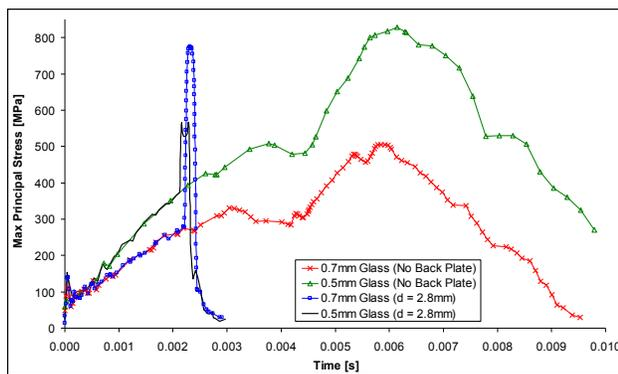
**Figure 8. Comparison of maximum principal stress for panels made with 0.7 mm and 0.5 mm thick glass sheets [3]. Also shown is a comparison between having a back plate at a distance of 2.8 mm from surface-4 and not having a back plate.**
