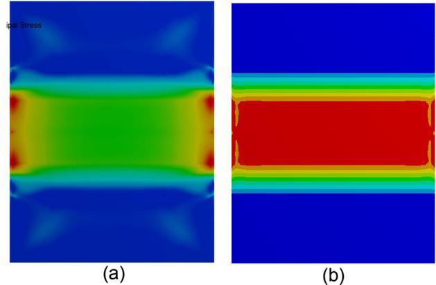
**Figure 4 [7-8]: (a) Stress distribution during a four-point bend test of a panel (surface-4 which is bottom of TFT glass is under tension); (b) Stress distribution during a four-point bend test of a monolithic glass of same size.**
