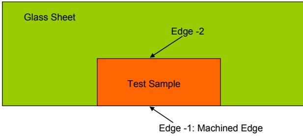
**Figure 5: If the objective is to find the strength of edge-1, then, only the samples that fail from edge-1 and which are inside the load-span should be used for reporting the strength.**
