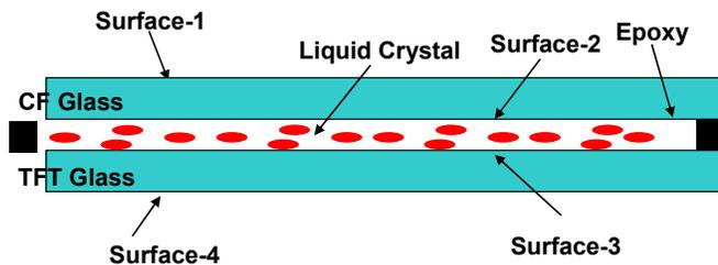
Figure 1. Notation used to refer to different surfaces in an LCD panel.
