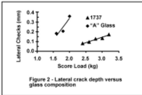
Supporting microscopic analysis was done that graphically illustrates the fundamental qualitative difference in how the two glasses fractured under the score load. The photos, figures 3 & 4, are 5000x SEM photo images of 1737 and A Glass, taken along the edge of a scored (2 kg load) and separated sheet. In glass A, substantial subsurface damage is generated during the score process, resulting in dramatic lateral cracking.
