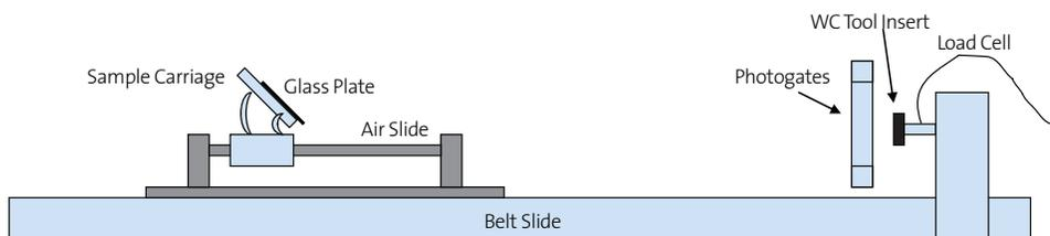
**Figure 1.** Impact test device
