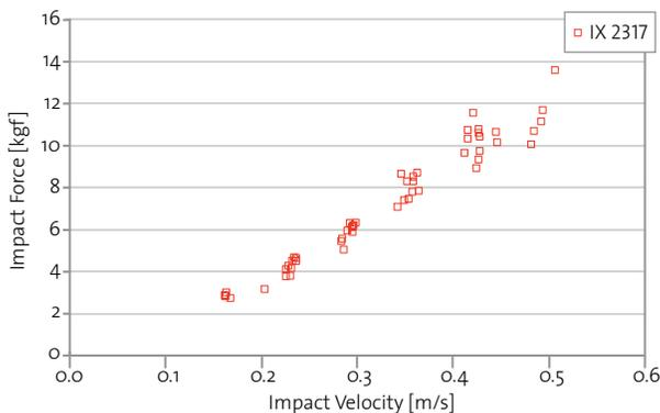
**Figure 5.** Impact force as a function of impact velocity for IX 2317
