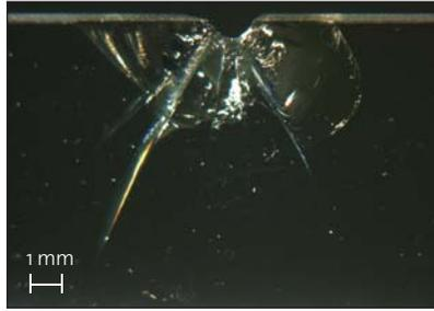
**Figure 3.** Crack system in NIX glass
