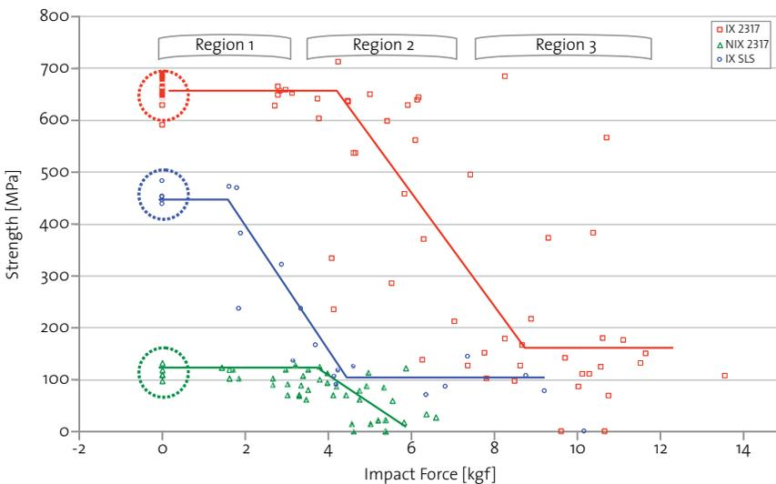
**Figure 6.** Retained strength as a function of impact force
