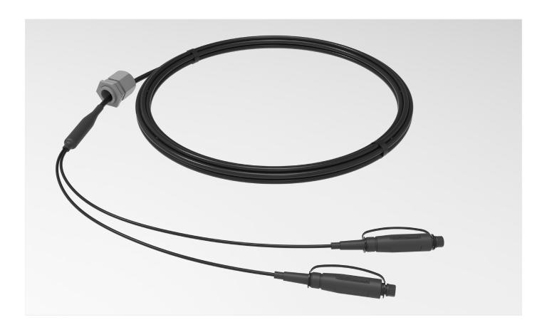
The Y Cable - 2-Fibre SST-Drop™ cable assembly with two factory-terminated, environmentally sealed and hardened OptiTap® connectors is designed to significantly reduce the cost and the time of drop cable deployment in optical access networks. It's self-supporting and is suitable for aerial, direct-buried or duct installation.
