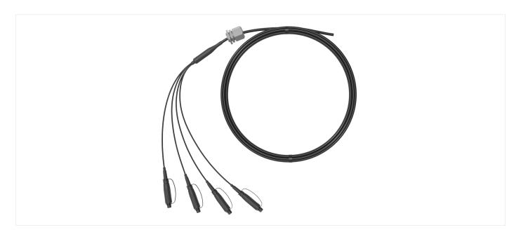
The X Cable - 4-Fibre SST-Drop<sup>®</sup> cable assembly with four factory-terminated, environmentally sealed and hardened OptiTap<sup>®</sup> connectors, is designed to significantly reduce the cost and the time of drop cable deployment in optical access networks. It's self- supporting and is suitable for aerial, direct-buried or duct installation.
