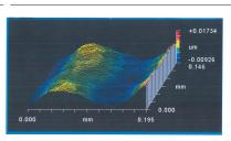
Smoothness of surface suggests primarily chemical removal during super-polishing ( lack of fracture surfaces).
