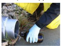
4. In areas where samples cannot be easily collected directly from the outfall, a decontaminated 500 mL polypropylene sample collection bottle attached to an extension pole can be lowered and/or extended to the desired sampling location.
