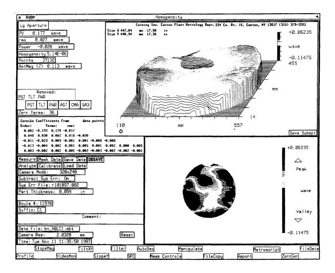
Figure 8. Index Homogeneity Measurements on Sub-scale Infrasil Part
