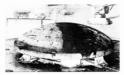
Figure 11. Convex Window Blocking Body on Corning Grinder
