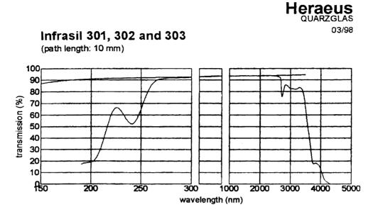
Typical spectral transmission including Fresnel reflection loss. The uppermost nearly straight line indicates the calculated Fresnel reflection loss of two uncoated surfaces.
