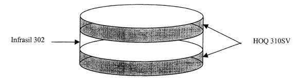
Figure 3. Stack Sealing of HOQ 310SV (top and bottom) with Infrasil 302
