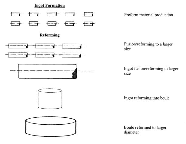
Figure 4. Forming Process to Produce 1.1 meter Boule of Infrasil
