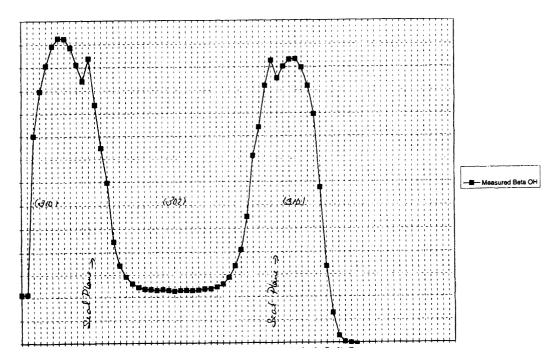
Figure 7. Beta OH vs. Distance for 6" Stack Seal of HOQ 310 and Infrasil 302
