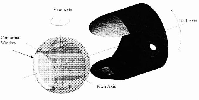
Figure 1. ABL Turret Assembly with Conformal Window
