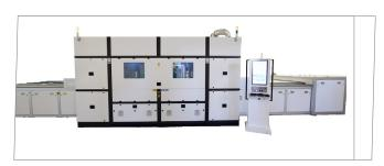
Using ultra-short laser pulses, the CLT 66G cuts by material disassociation rather than ablation. The result is a very low surface roughness, increased as-cut edge strength and yield.
