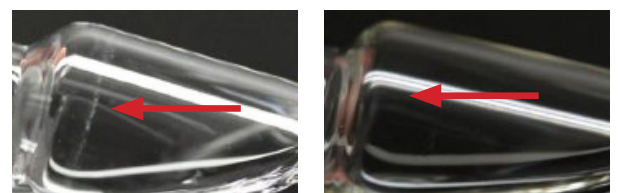
Visible scratches are less evident after pharmaceutical processing with Valor glass vials (right) compared to conventional borosilicate containers (left).
