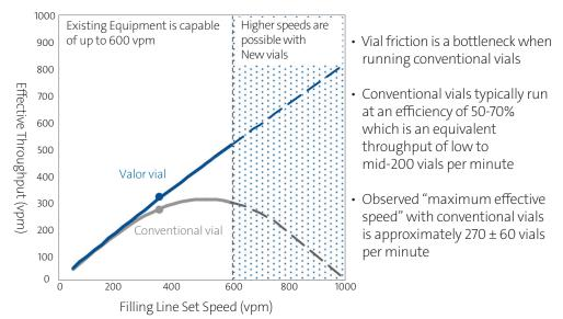
Valor vials can maintain high efficiency (>80%) at higher filling line set speeds
