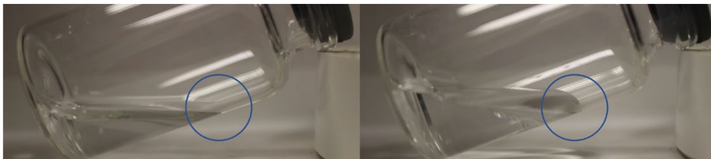
Figure 2. Glass vials with water showing perfect wetting (left) and de-wetting (right) behavior.
