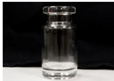
Figure 6. Steps in a wetting assessment. At left, a horizontal vial is filled with water then rotated to initially wet all surfaces. At right, the vial is stood upright and the behavior of the meniscus is monitored.
