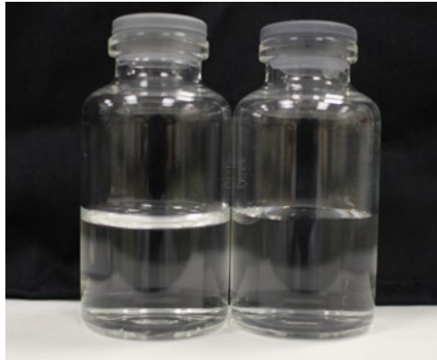
Figure 4. Glass vials with high purity water showing uniform wetting (left) and uniform de-wetting (right).
