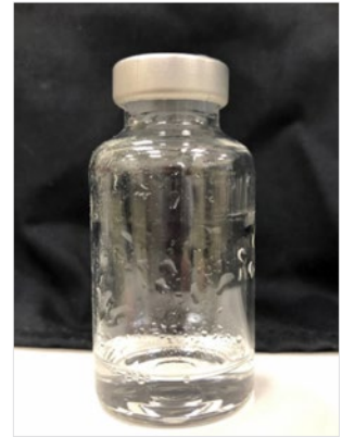
Figure 5. Non-uniform wetting and de-wetting behavior in a glass vial headspace.
