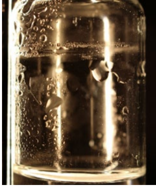
Figure 7. Glass vial exhibiting non-uniform wetting in defined rings or bands around the vial and isolated areas. This was produced by filling a depyrogenated glass vial with water and closing with an elastomeric stopper and aluminum cap, then terminally sterilizing (60 minutes at 121°C).
