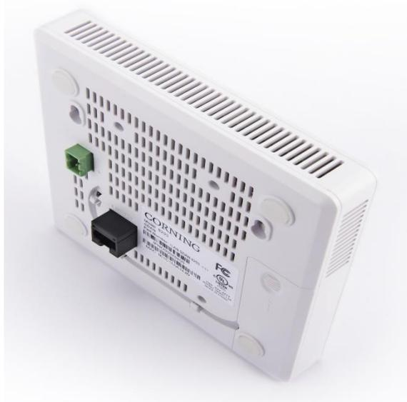
Model 1 LAN-ONT-8293 Rear View showing 3<sup>rd</sup> Ethernet port and power connection from the back side of the unit
