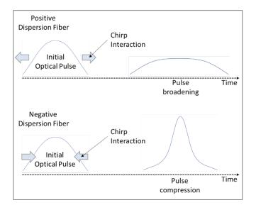
Figure 2: Chirp Interaction on Optical Pulse
