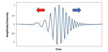
Figure 1: Positive Frequency Chirp (Up-Chirp)
