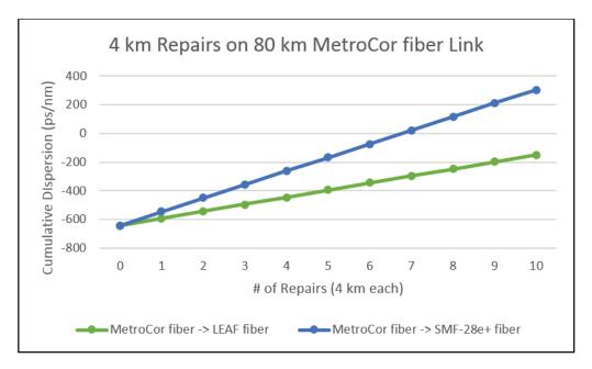
Figure 4: LEAF Fiber and SMF-28e+ Fiber Repairs on MetroCor Fiber Link
