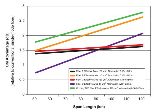
Figure 2. Corning TXF fiber performance advantage compared to other single-mode fiber designs targeted at terrestrial long-haul.
