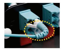
Figure 5. Pull connector as a result of entropy effect over time
