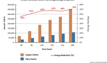
Figure 3. Energy savings comparison of fiber vs copper based systems
