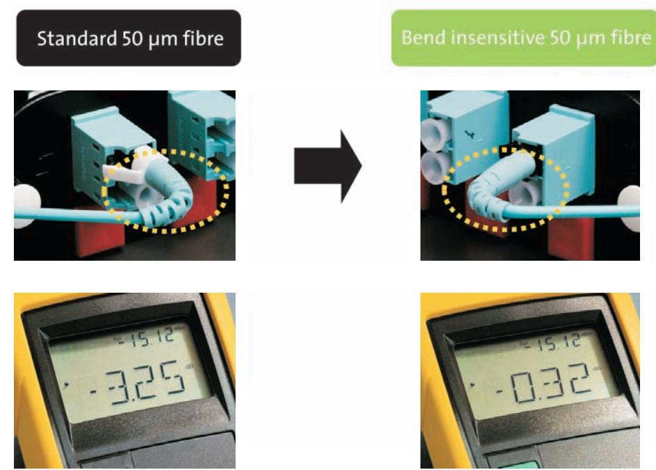
**A single tight bend can cause a signal loss of over 3 dB, that's a 50% power reduction:
