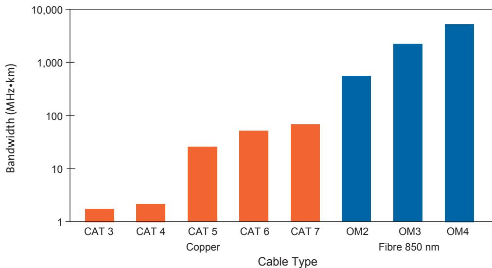
**Bandwidth comparison of copper\* and fibre\*\* cables. OM2 fibre bandwidth capability has outlived all generations of copper cable design; OM3 and OM4 bandwidth and link length capabilities are even further beyond that of copper. \*Bandwidth frequencies for copper are typically referenced to 100m, here they are normalised to 1km.**
