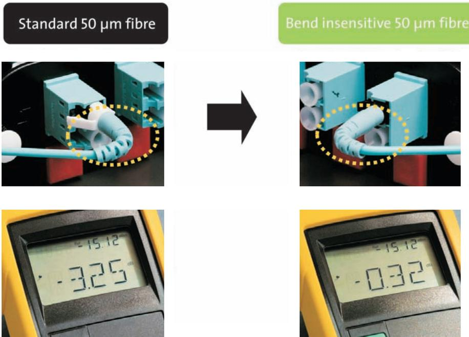
**A single tight bend can cause a signal loss of over 3 dB, that’s a 50% power reduction: such power loss would cause a 10 G link to fail! A bend insensitive multimode fibre under the same condition will exhibit 10 times less loss and so maintain a strong signal and no link failure.**
