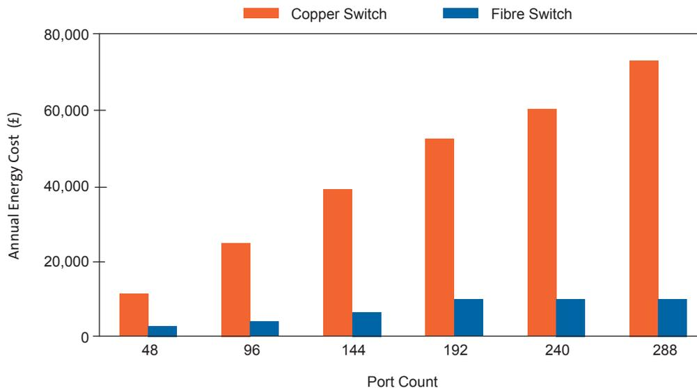
**Comparison of the total electronics and cooling energy cost of 10GBASE-SR optical and 10GBASE-T copper**
