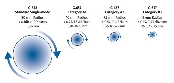
Figure 4. Tightest Bending Conditions Specified by the Different Fiber Categories of ITU-T Recommendation G.657 Compliant Optical Fiber
