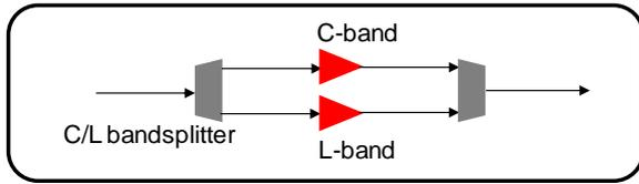
**Fig. 2: Illustration of amplifier configuration in one direction for C+L system.**
