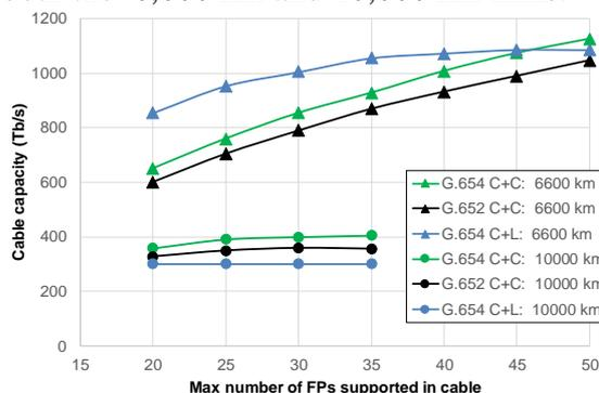
**Fig. 9: Theoretical cable capacity as a function of maximum number of fiber pairs built in cable.**
