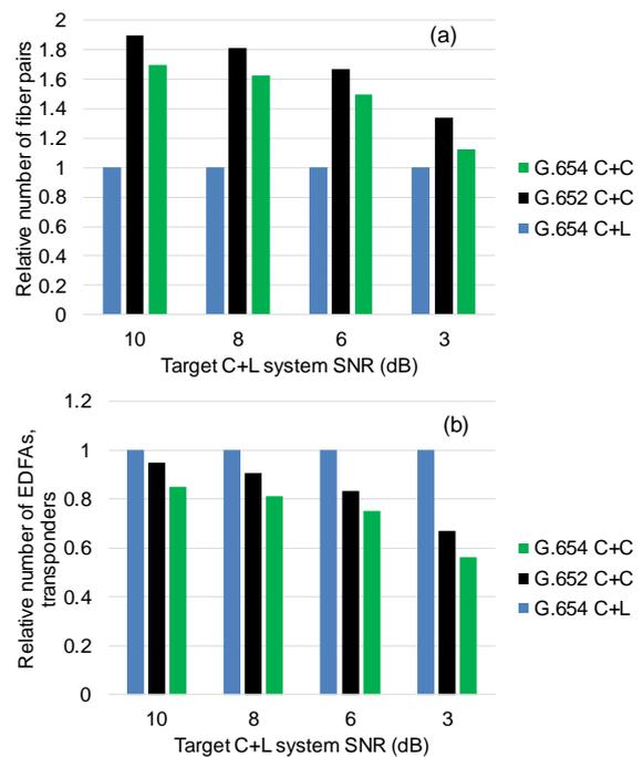
**Fig. 5: 6,600 km link with 60 km spans. a) Relative number of fiber pairs required to achieve equal capacity. b) Relative number of transponders and EDFAs required.**
