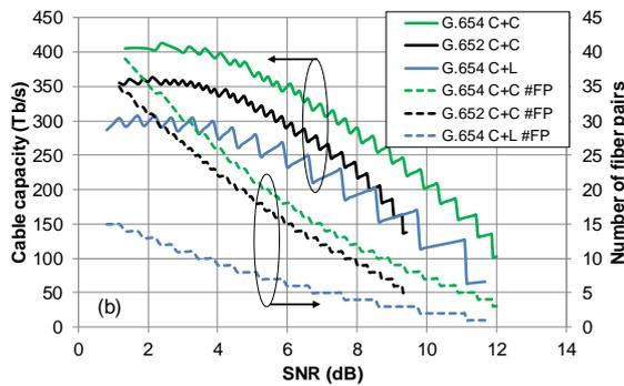
**Fig. 3: Cable capacity and number of fiber pairs vs. SNR for a) 6,600 km system, and b) 10,000 km system.**
