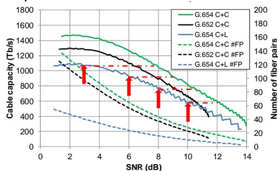
**Fig. 4: Cable capacity and number of fiber pairs vs. SNR for 6,600 km system with four capacity levels illustrated.**
