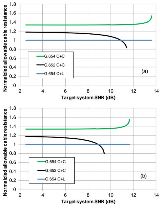
**Fig. 8: Relative allowable cable conductor resistance for equal capacity systems with same target SNR values for link lengths of a) 6,600 km and b) 10,000 km. The span length for all systems is 60 km.**
