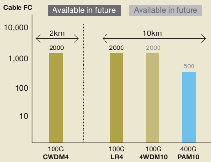
Figure 3: Fibre counts needed to achieve 100Tb/s transmission
