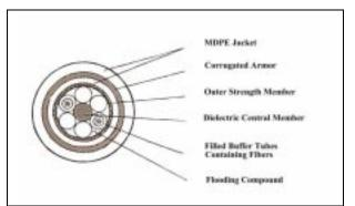
Figure 1. Loose-Tube Cable Structure
