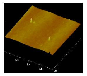
Figure 6: AFM scan of field-aged fiber with surface roughness of 0.29nm
