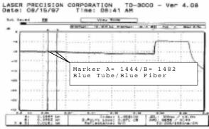
Figure 2: OTDR trace of fiber distance marking
