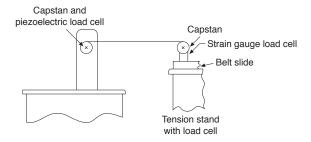
Figure 1 Schematic drawing of the belt slide tensile testing apparatus.
