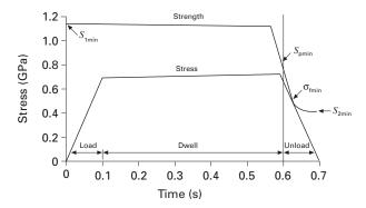
Figure 7 Schematic drawing of a typical proof test event.
