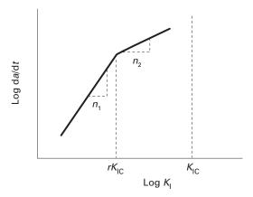
Figure 5 Schematic drawing of the two-region power-law model.
