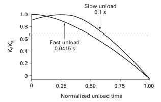
Figure 8 Dependence of the stress intensity factor on unload time for various unloading cases.
