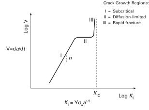
Figure 4 Class K-V curve for silica glass.
