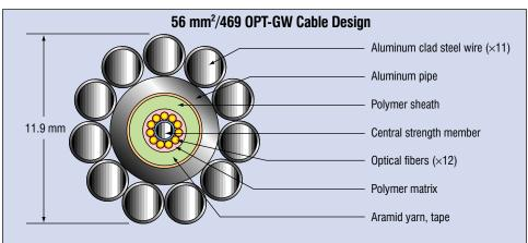
**Fig. 1.** This diagram depicts the 56 mm<sup>2</sup>/469 optical ground wire used for the test. The nomenclature 56 mm<sup>2</sup>/469 refers to the cross-sectional area of the stranded aluminum-clad steel wires (56 sq mm) and the outer diameter in thousandths of an inch (0.469 inch).
