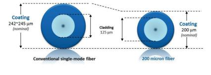
Cross sections of conventional and 200-micron fibres
