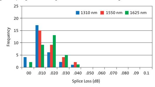
Core Alignment Splicing: Reduced coating diameter fiber vs convention coating diameter fiber w/ similar MFD
