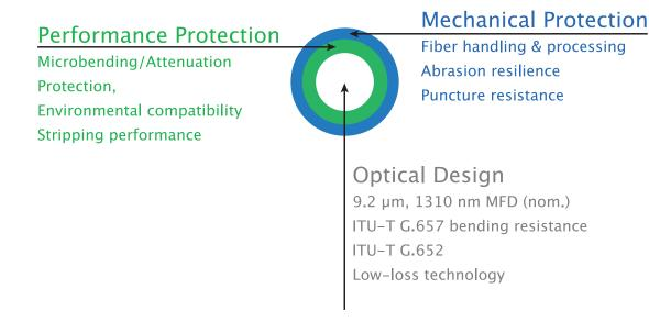
Figure 1. Two main principle functions of the dual-layer Corning CPC<sup>®</sup> protective coating and key design aspects of the central glass fiber.
