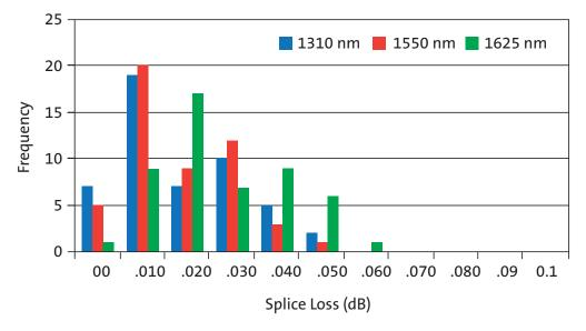
Figure 4. Representative splice loss of ITU-T.G652.D reduced diameter fiber spliced to itself.
