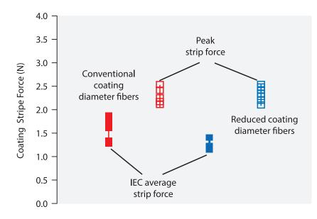
Figure 3. Comparison of coating stripe force: Conventional vs. reduced coating diameter fibers.
