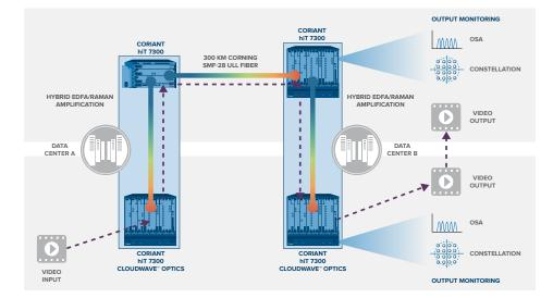
Coriant and Corning Team to Demonstrate Low cost, High Capacity DCI Transmission with the Powerful Combination of Coriant CloudWave<sup>™</sup> Optics and Corning<sup>®</sup> SMF-28<sup>®</sup> ULL Optical Fiber
