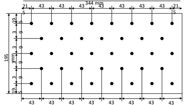
**Figure 2. LED grid layout for the ultra-slim BLU prototype.**
