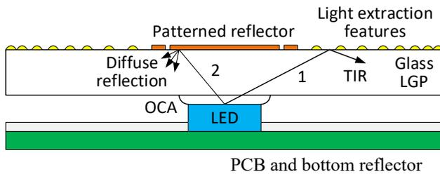
**Figure 1. Schematic of an ultra-thin BLU cross-section segment near one of the LED sources.**
