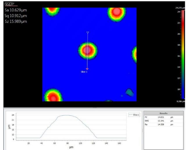
**Figure 3. Zygo interferometer measurement results for a single droplet of white ink on glass.**
