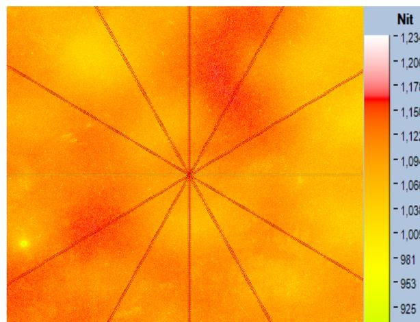
Figure 5. False color luminance map of approximately 86 x 76 mm area in the center of backlight.
