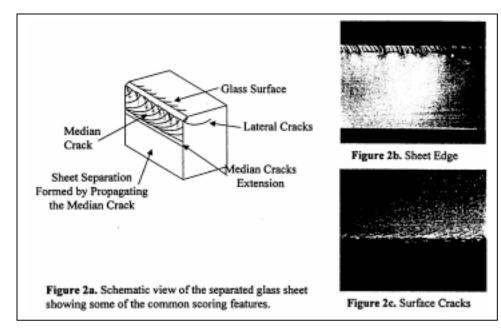
Figure 2a is an isometric sketch of a scored and separated sheet, labeled with most of the critical features found on a typical edge.
