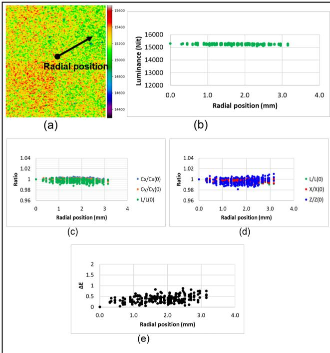
**Figure 3. (a) Measured 2D spatial luminance distribution; (b) Luminance vs. radial position; (c) Ratios of  $C_x/C_x(0)$ ,  $C_y/C_y(0)$ , and  $L/L(0)$  vs. radial position; (d) Ratios of  $L/L(0)$ ,  $X/X(0)$ , and  $Z/Z(0)$  vs. radial position; and (e)  $\Delta E$  vs. radial position.**
