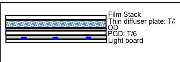
**Figure 2. PGD based mini-LED backlight including a light board, a PGD of thickness  $T/6$ , a QD film, a thin diffuser plate of thickness  $T/3$ , and a film stack.**
