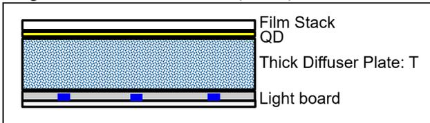
**Figure 1. A reference mini-LED backlight including a light board, a thick plastic diffuser plate of thickness  $T$ , a QD film, and a film stack.**
