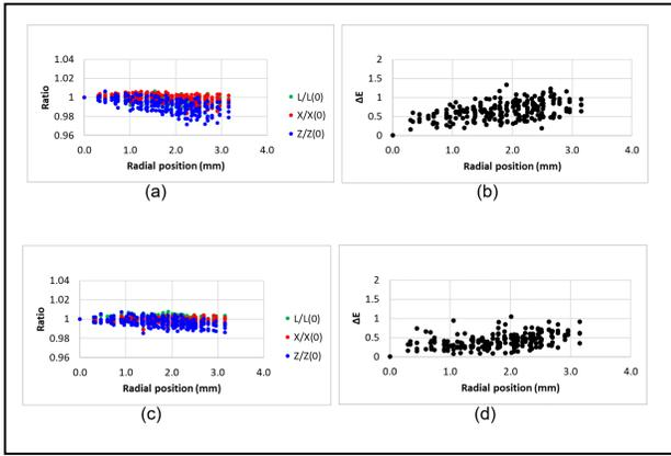
**Figure 4. Measured zone uniformity over the reference mini-LED backlight including a thick diffuser plate of thickness  $T$ . (a) Ratios of  $L/L(0)$ ,  $X/X(0)$ , and  $Z/Z(0)$  vs. radial position for film stack 1; (b)  $\Delta E$  vs. radial position for film stack 1; (c) Ratios of  $L/L(0)$ ,  $X/X(0)$ , and  $Z/Z(0)$  vs. radial position for film stack 2; and (d)  $\Delta E$  vs. radial position for film stack 2.**
