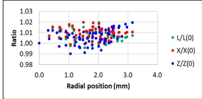
**Figure 5. Simulated ratios of  $L/L(0)$ ,  $X/X(0)$ , and  $Z/Z(0)$  vs. radial position.**
