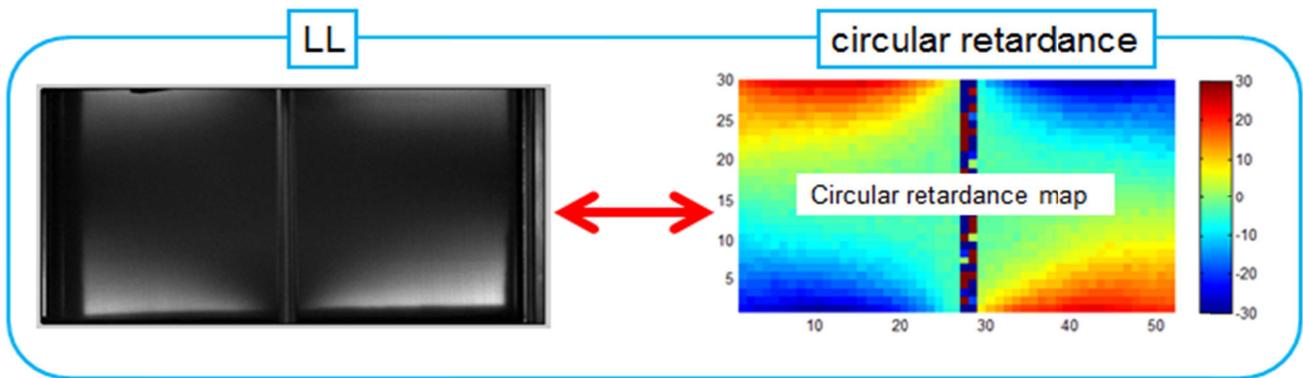
Figure 2. CCD image of curved IPS panel LL in dark state (left) and measured circular retardance with analyzer removed.
