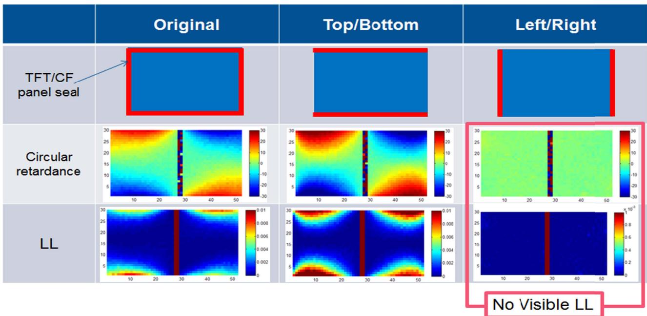
Figure 3. Curved IPS panel with original seal, left/right and top/bottom seal removed vs. measured circular retardance and LL. The vertical band in the center of the figures in the lower two rows is an artifact from the fixture holding the panel.
