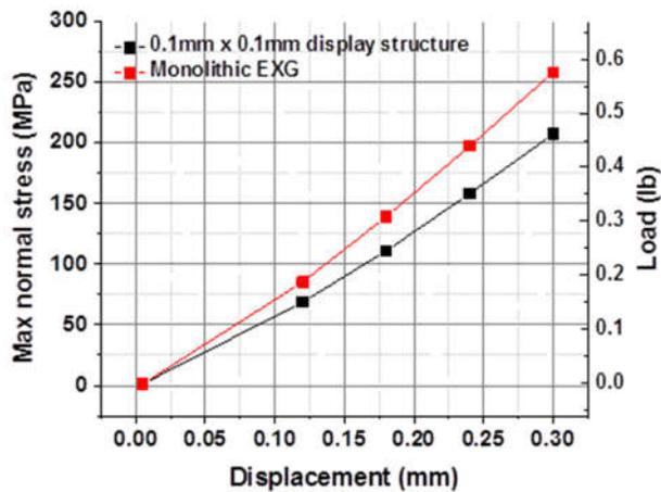
Figure 5. Stress and force vs. displacement curves for ESMS measurement simulations using FEM.
