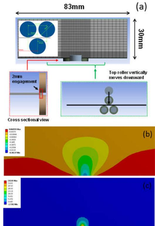
**Figure 4.** (a) Geometry used for FEM analysis. Compliant (durometer ~ 70 shore) polyurethane compound. Diagram showing roller dimensions is flipped relative to other drawings. (b) Panel displacement of the surrounding measurement region (~30µm displacement in immediate tensile zone). (b)Stress field corresponding to displacement in 2b (maximum stress ~ 240MPa).
