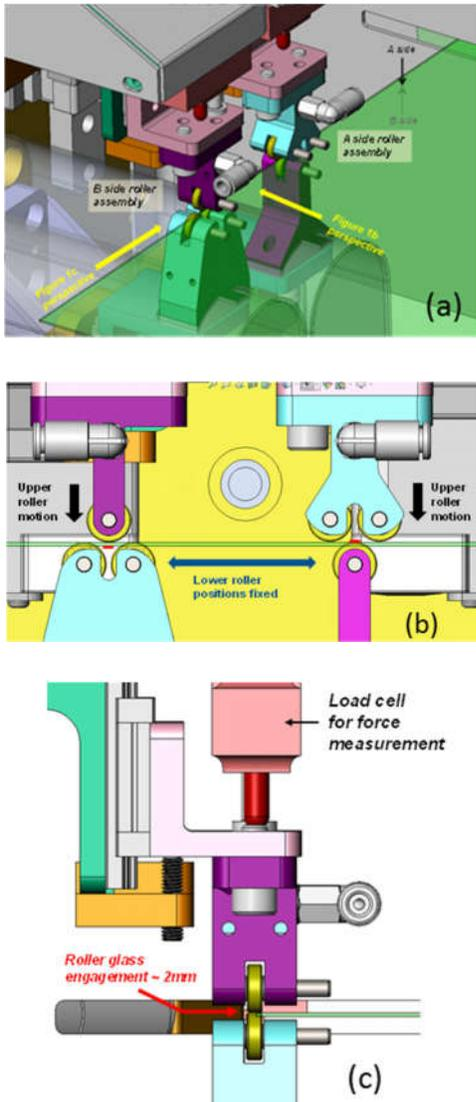
**Figure 3.** (a) Isometric depiction of the ESMS roller heads engaged with a sheet of glass. A side and B sides are labeled accordingly with visual aid markers for parts b and c. (b) Rollers engaged with the glass from normal perspective. Roller motion profiles and positions are indicated. Red lines indicate regions of tensile stress application. (c) Tangential view of roller engagement. The out-most 2mm of the edge are engaged with the roller surfaces.
