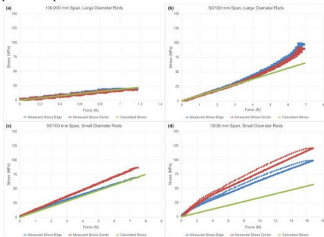
**Figure 1. Stress vs force for a variety of given configurations: a) large rods, 100/200 mm test span, b) large rods, 50/100 mm test span, c) small rods, 50/100 mm test span, d) small rods, 18/36 mm test span. All show an inability to generate sufficient stress before a 50 mm deflection.**
