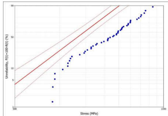
**Figure 2. Weibull plot for a simulated measured data set (blue dots) with Weibull prediction curve after an area correction factor (red line). Lighter red lines indicate reliability bounds for the Weibull prediction.**
