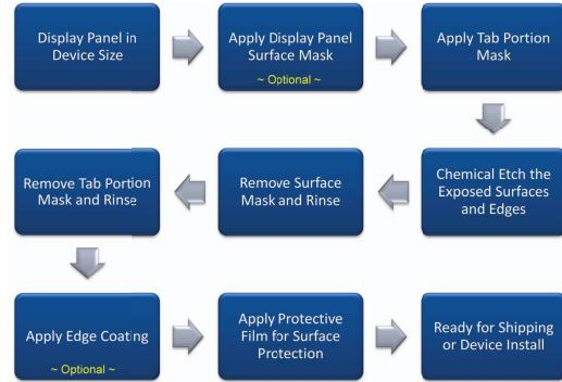
**Figure 7. General process flow for strengthening a device level display panel.**
