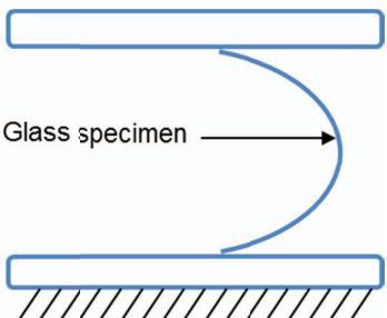
**Figure 5. Schematic of two point bend test.**
