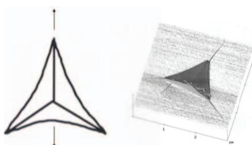
**Figure 1. Atomic force microscopy of a 1 gram indent from a cube corner indenter. [2]**
