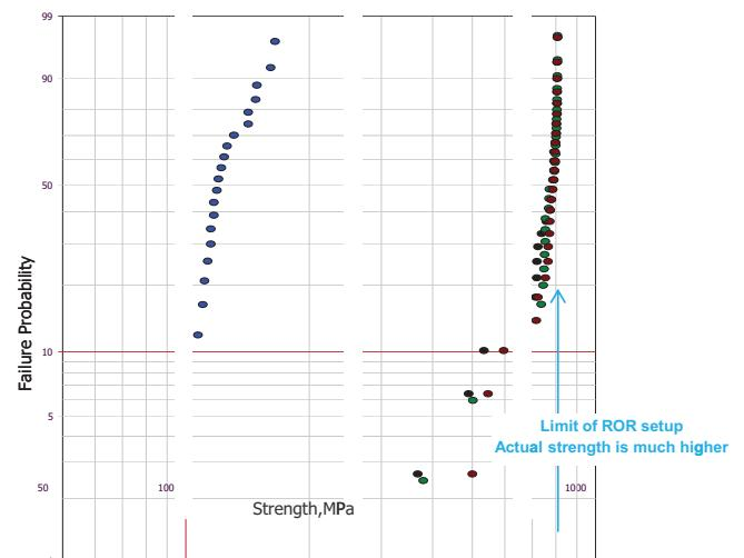
**Figure 4. Surface strength of specimens using ring-on-ring test.** 800 MPa was the limit of the test setup and so the actual strength is much higher.
