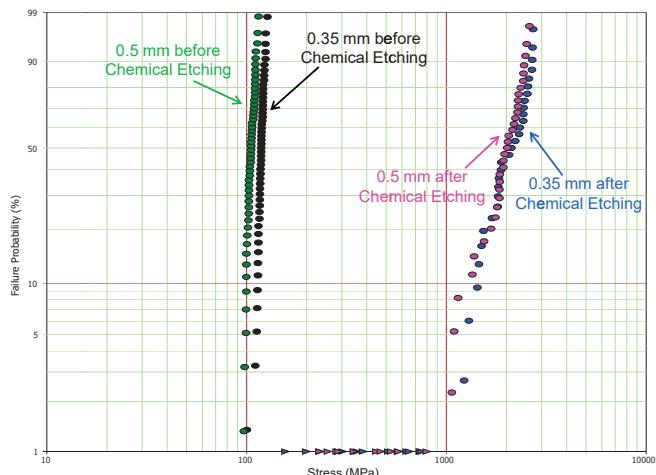
**Figure 6. Two-point-bend testing of score/break specimens with score-side in tension.**
