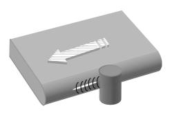
Fig. 12 Schematic illustration of the identified mechanism of origin creation on the case. The glass sheet slides in the direction of the arrow against the fixed pin, and the relative rubbing direction by the pin is in the opposite direction (left to right in this figure).
