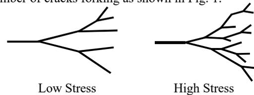
**Fig. 1 Forking with high and low stresses.**
