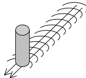
**Fig. 3. Schematic illustration of relation between friction direction and shapes of Chatter marks. Drawing shows that the glass is stationary and the object is moving in the direction indicated by the arrows.**
