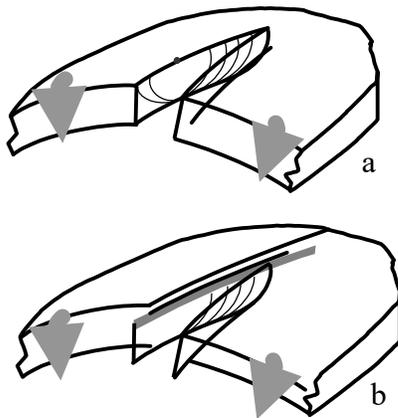
**Fig. 13. Schematic illustration of (a) breakage and (b) cutting. The only difference between (a) and (b) is the origin of crack propagation. Irregularly created damage as origin for breakage (a) and median cracks created with scribing as controlled origin for the cutting (b).**
