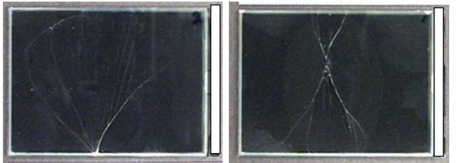
**Figure 6. Typical forking pattern (a) Failure origin on the edge; (b) Failure origin on the surface.**
