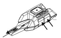
**Step 9:** Hold scrap fiber and press Red button to remove.
