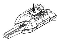
Step 8: Remove fiber from handler and check cleave length against guide.
