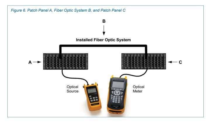
NOTE: The procedure to reference an OLTS/LSPM can be different from one test equipment manufacturer to another. Please refer to the specific manufacturer's test equipment reference methods to ensure the test equipment is referenced correctly.
