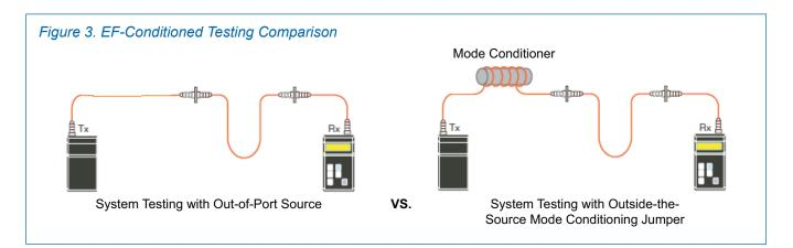
Corning believes that EF is the most accurate method to test multimode fiber. An EF-conditioned launch will reduce the variability among sources today (+20/-40 percent) to the respectable +/- 10 percent variability, and it will provide the best system characterization for 1 Gb/s and beyond.
