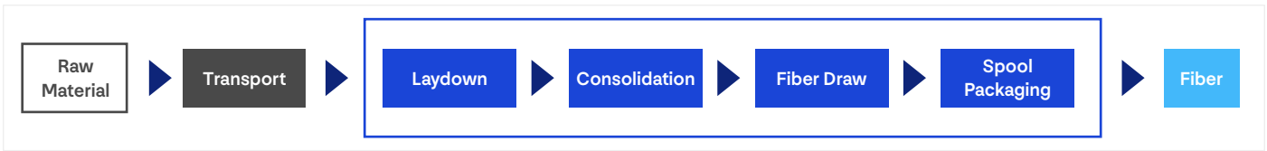
Figure 3. Process flow of the significant manufacturing stages of the optical fiber
