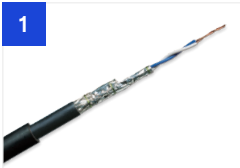
CCXSCB-LB047-C003-L7 S/FTP, 1200 MHz, AWG22, Cat.7 A , 4P Simplex, B2ca, s1a, d1, a1, up to 120 m with KS500S Jack
