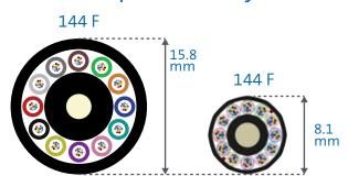
50% smaller than loose tube cables
