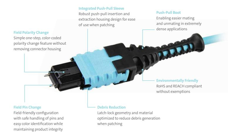
Our industry-leading MTP° connector family has a new addition – the MTP° PRO connector with push-pull boot. Now standard on all FDGF® and FDGF8° assemblies.\*
